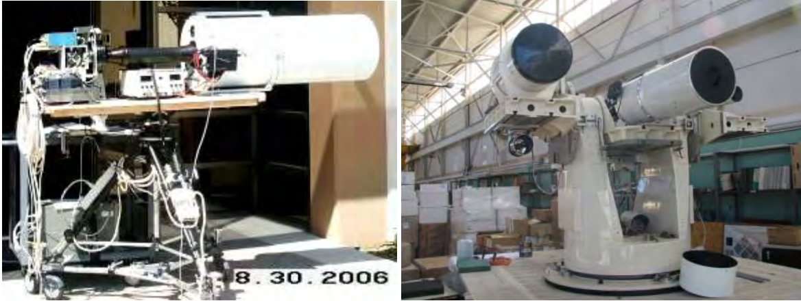
Figure 8b. The InSb VariAp® camera with the relay optics, correcting lens and a Ritchie-Chretien 12.5" telescope (left), and the system on a tracker mount at WSMR (right).
