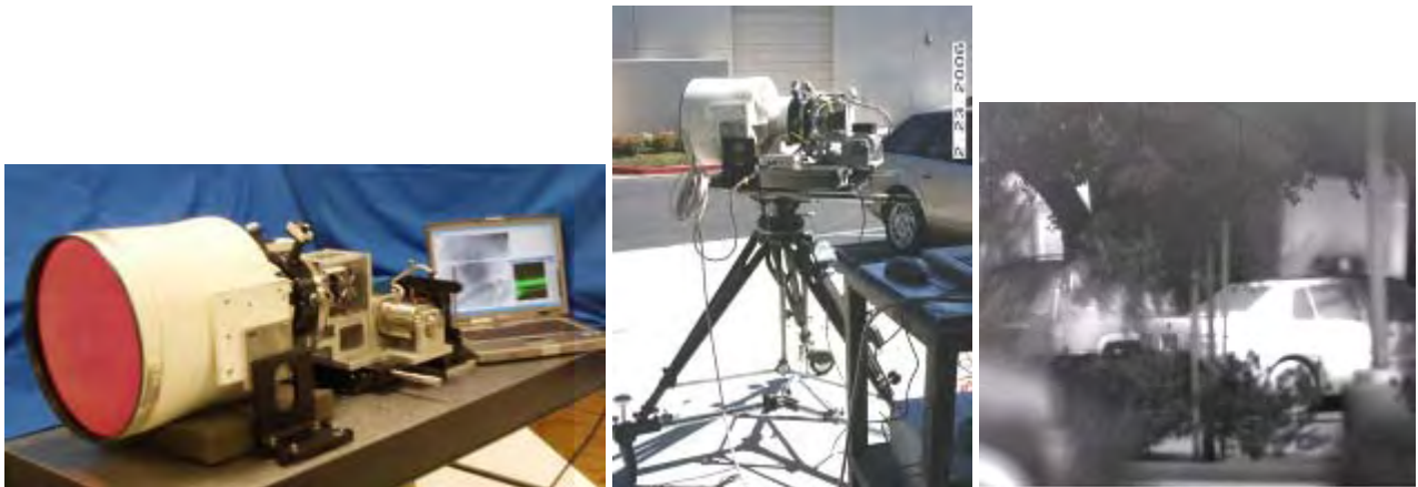
Figure 8a. The InSb VariAp® camera with a 500 mm, f/1.67 refractive lens, and an image captures with the system.
