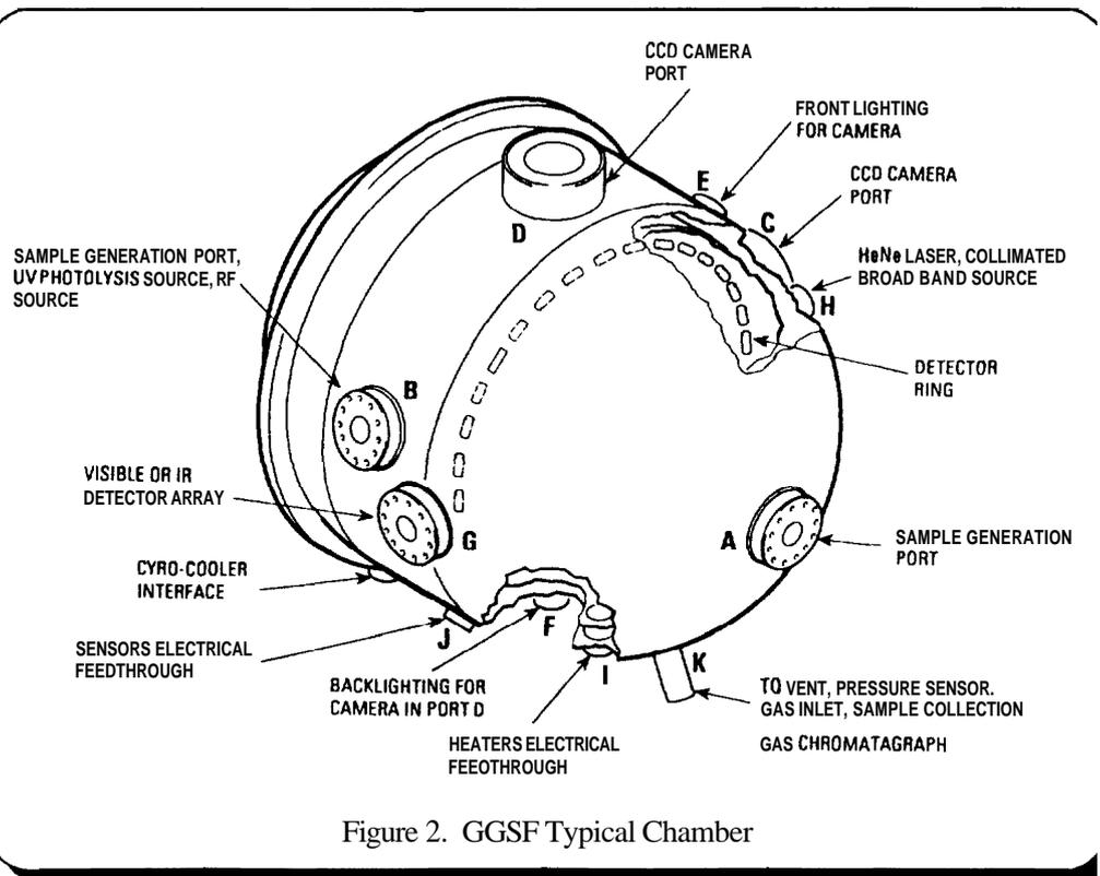
Figure 2. GGSF Typical Chamber
