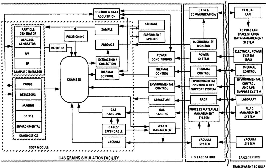
Figure I. GGFS Block Diagram and SSF Interfaces
