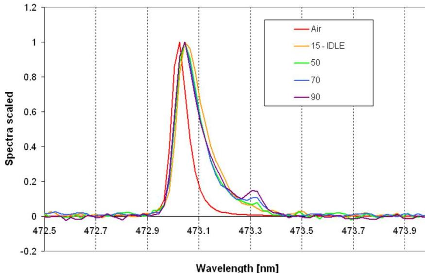
**Figure 6. Normalized CARS spectral measurements acquired during J85 engine operations ranging from idle to military PLA conditions.**
