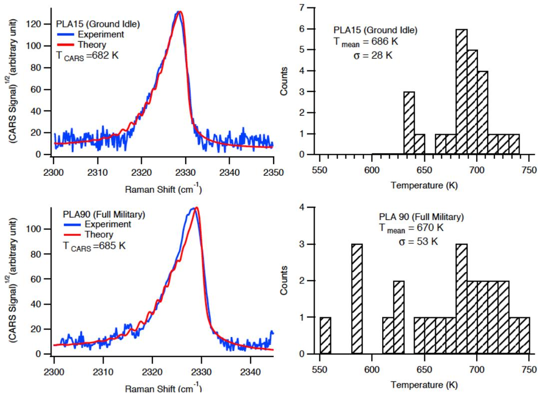
**Figure 11. Plot (left): 20-shot-average nitrogen vibrational CARS spectrum taken in the exhaust of the J85 at PLA 15 and PLA90 compared to theory. Probability Density Function (right): Corresponding temperature PDFs for 25 consecutive 20-shot-average CARS spectra.**
