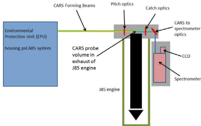
**Figure 8. Schematic view of ps-CARS experimental setup at the PRF/J85 site.**
