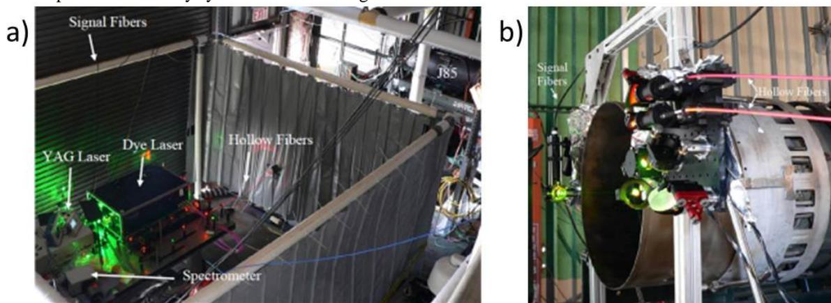
**Figure 3. Photographs of the ns-HCWG CARS system during test demonstrations at the PRF facility. a) overhead photograph showing the laser system installation in relation to the J85 engine, b) photograph of the beam-delivery optics (foreground) and signal-collection optics (background) located downstream of the J85-engine nozzle exit plane.**
