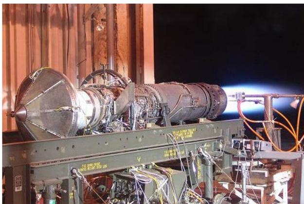
Figure 1. GE-J85-5 engine mounted on an A/M37-T20 thrust stand in the PRF facility.
