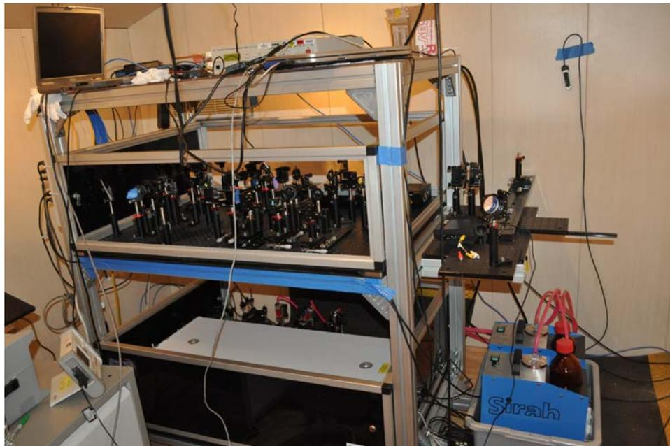
**Figure 9. Photograph of the transportable ps-CARS system installed inside the EPU at the PRF/J85 site.**
