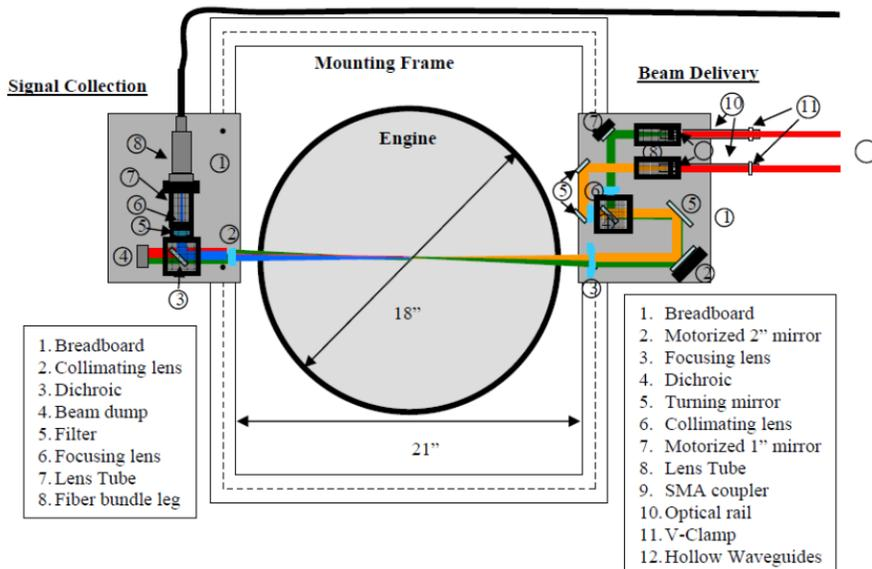
**Figure 5. Schematic diagram of the experiment setup, aft looking forward.**
