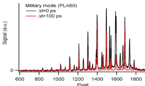
**Figure 13. Single-shot spectra (corrected for dark counts) acquired during J85 engine operations at PLA 60 and a probe delay equal to 0 (back) and 100 ps (red).**
