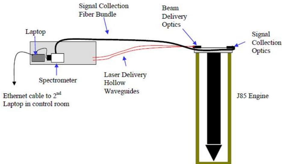
**Figure 4. Schematic diagram of the ns-HCWG experimental setup at the PRF J85 site (not to scale).**
