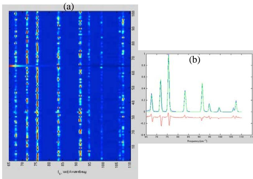
**Figure 15. (a) Distribution of 100 single-shot RCARS spectra. (b) Fitted experimental 100-shot-average spectrum acquired at room-air condition and delay equal to 100 ps.**
