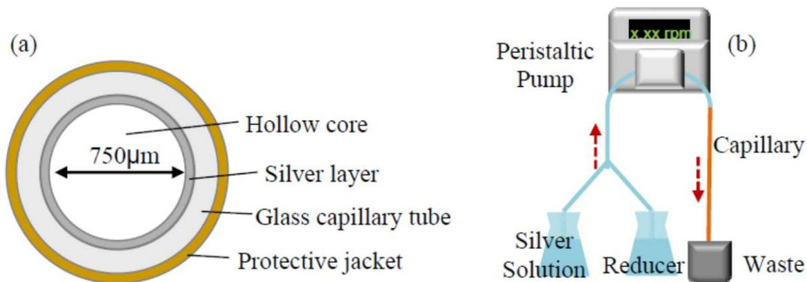
**Figure 2. (a) Diagram of a silver-coated HCWG and (b) simplified schematic illustrating the method for applying silver coating to the inside of a glass capillary tube.**
