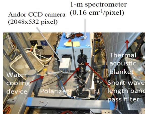
**Figure 10. Detection system for CARS signal.**
