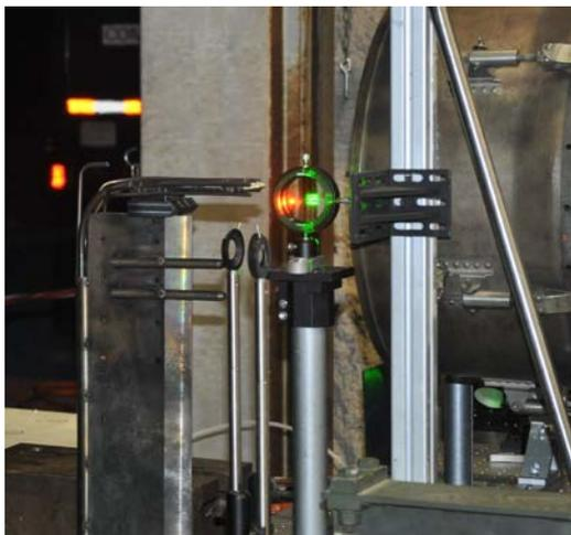
**Figure 12 - Photo of two-beam ps-RCARS setup J85 engine exit plane.**
