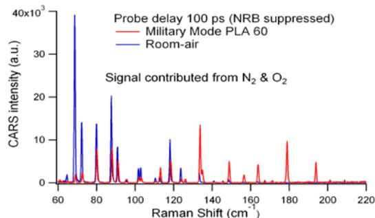
**Figure 14. Single-shot spectra for room air conditions (blue) and the J85 engine operations at PLA 60 g (red).**
