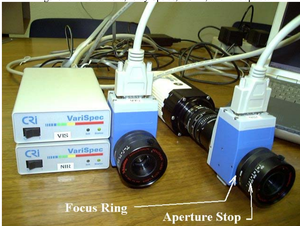
Figure 2. Each LCTF has a dedicated controller box (same serial numbers).
