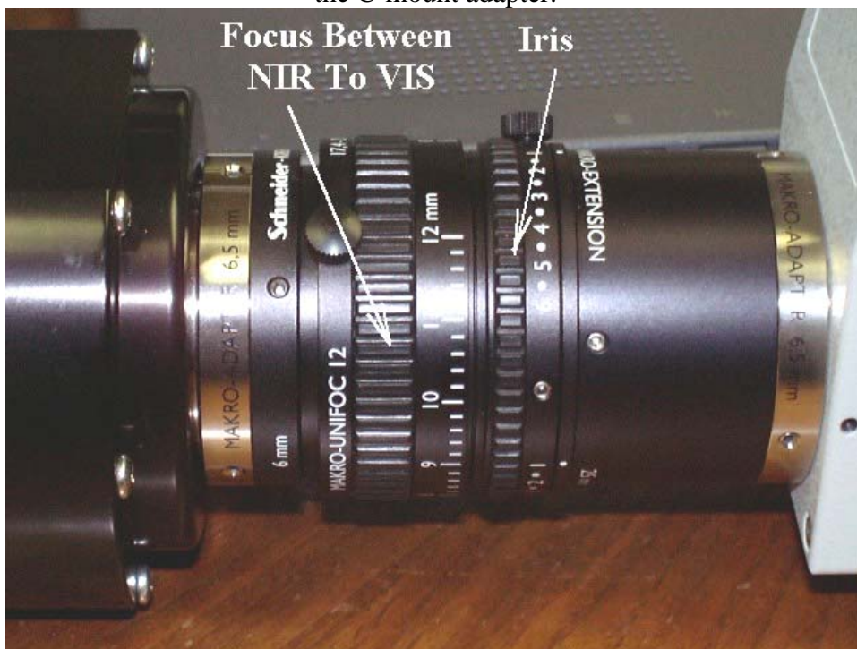
Figure 4. When switching between the VIS & NIR LCTFs use the focusing ring on the relay optics to focus the image (the difference between VIS and NIR is about 2 mm motion). Make sure that the front lens is focused to infinity (all the way in the FAR direction). Lock this focusing ring in place and use the front lens to focus to close by objects.
