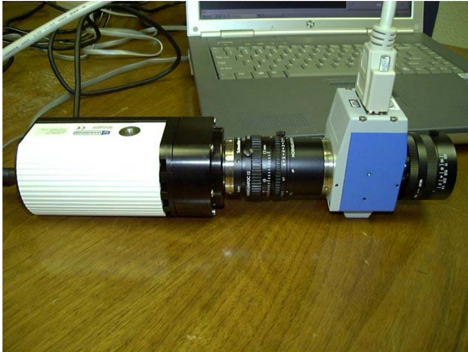
Figure 1. The camera, relay optics, LCTF, and foreoptics.
