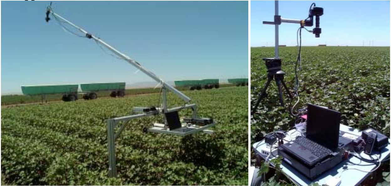
Figure 8. Precision farming; crop canopy spectral signatures measurement in support of remote sensing.
