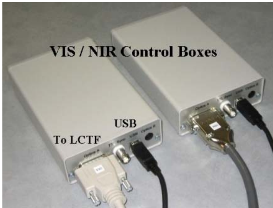
Figure 7. The two LCTF control boxes have identical connections for USB cables and the optics.
