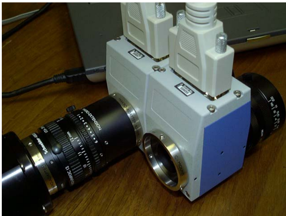
Figure 3. To switch from one LCTF to another, use the 3 set screws in the back of the LCTF, on the C-mount adapter.
