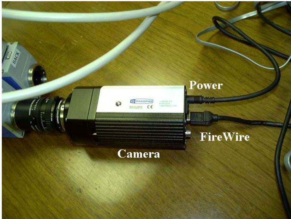
Figure 5. The camera has two connectors: power and FireWire. The power switch should be turned to “aux”.
